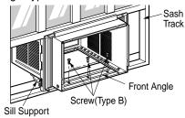
Step 8. Pull the frame curtains to each window sash track. Attach them on each side to the window sash and the window stool using 4 type C screws.
